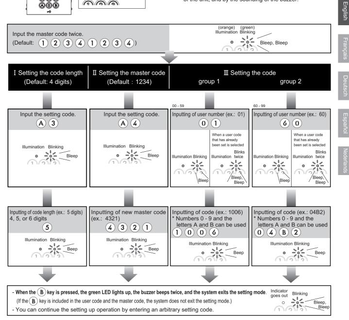
The set code will be saved in memory, even if the code length is changed. However, codes of different lengths cannot be used.
