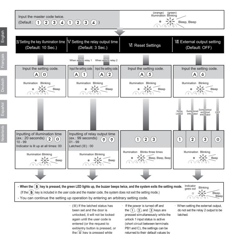
turning the power back on and pressing the (1), (2), and (3)
