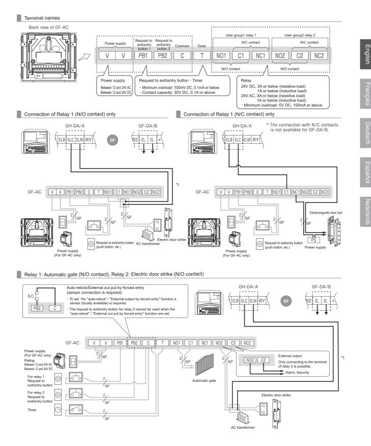
(\*1) The relay operating time of GH-DA/A (GF-DA/B) is different from that of GF-AC.
